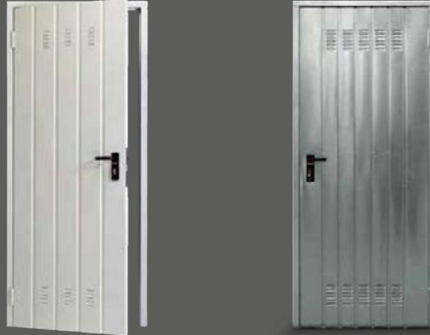
*It is made entirely in pressed galvanised steel strengthened with internal omega-shape reinforcement that make it non-deformable. It can have the opening to pull or push, with shutter left or right. It is supplied complete with handle and lock for closing both from inside and outside. Available on all the colors of the De Nardi RAL range.*
